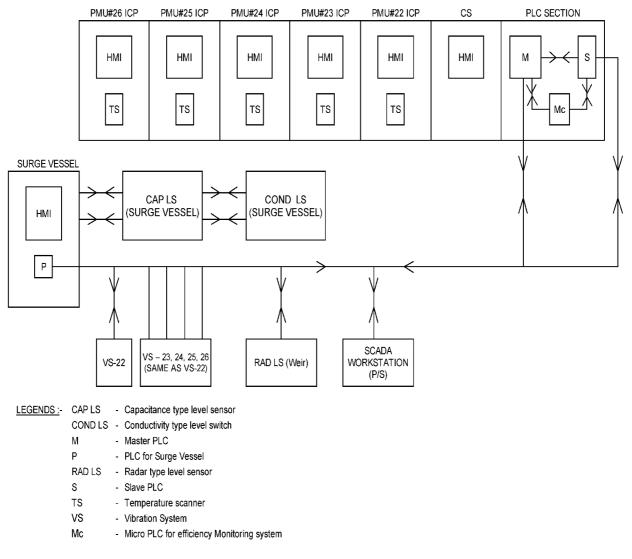
BLOCK DIAGRAM OF PLC AND SCADA SYSTEM (M-3 A PUMPING STATION, PISE)
