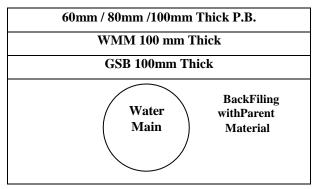
B) Cross Section for Reinstatement of Trenches in Asphalt
