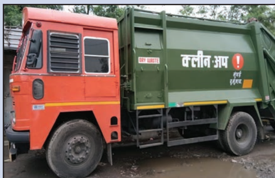
Compactor with Additional Chamber of Dry Waste Garbage
