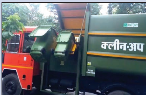
Compactor with separate chamber for collection of Dry waste and E waste
