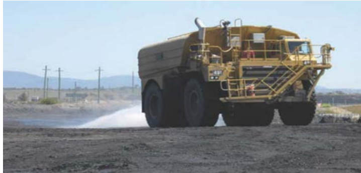
Figure 1 : Road side sprinkling of dust control agents
