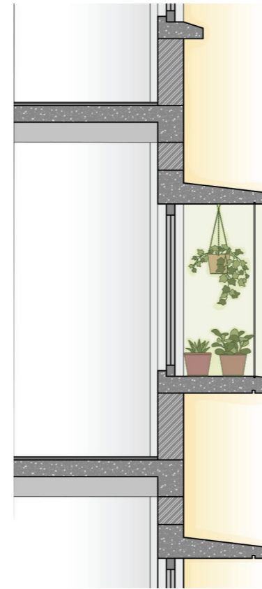
Figure 2.2: Container planting in windows with grills projecting externally at sill level.
