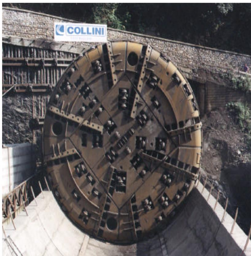
Tunnel Boring Machine
