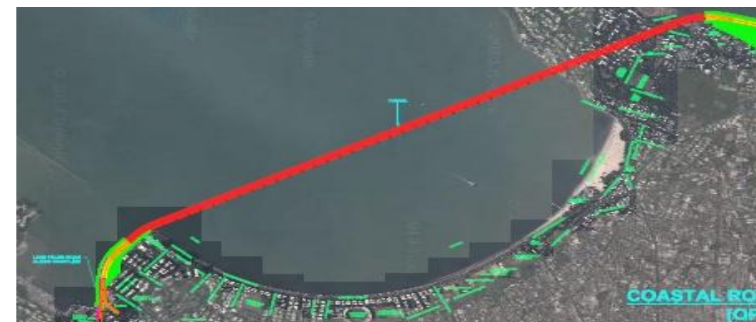
Figure 8.2 Proposed Tunnel Alignment
