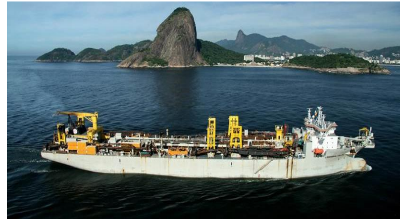
Figure 4-11 Jan De Null's Cristóbal Colón - Hopper capacity 46,000m 3
