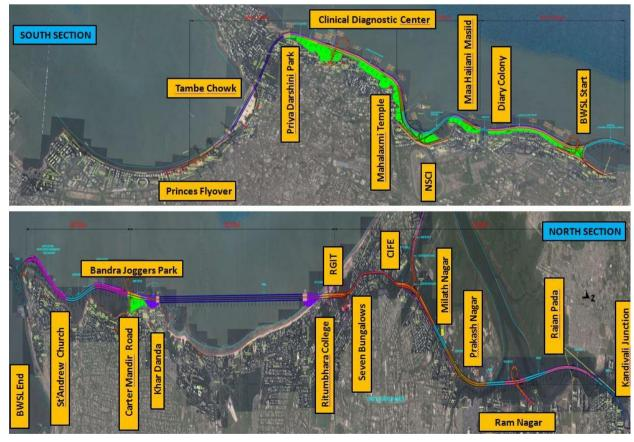
Figure 2.1: Alignment of the Proposed Coastal Road
