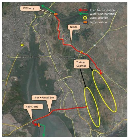
Figure 2.28: Transportation Plan from Turbhe Quarry
